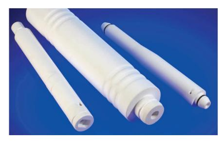
Larger hydrocyclone liners can be custom built in multiple sections using specially formulated joint technology. Proven for lengths up to 1.2m and internal diameters up to 250mm, the technology is scalable to larger sizes where requested.
