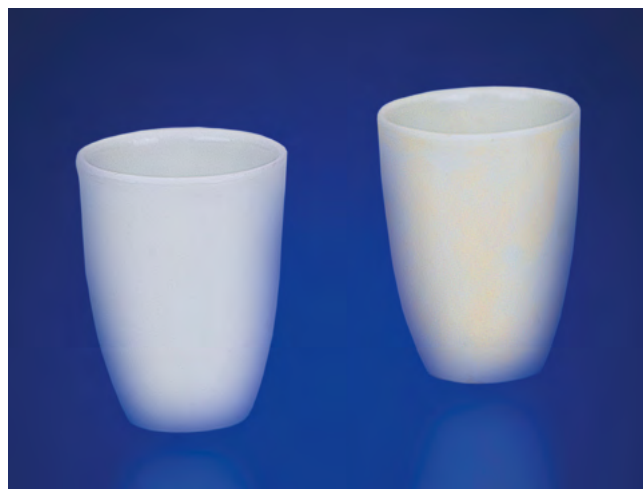
Competitor crucibles shown before (left) and after (right) anneal testing. Significant discoloration can be detected after the first anneal cycle.
